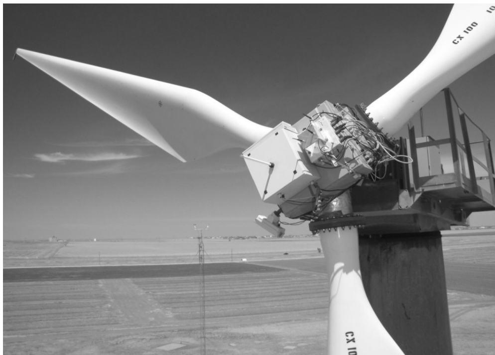
Figure 9: Sensor Blade 1 mounted on a test turbine at the SNL and USDA-ARS wind energy technology test facility in Bushland, TX
