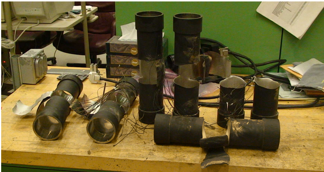
Fig. 7. Specimens failed under various thermomechanical loading conditions
