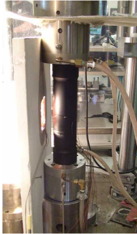
Fig. 2. Thermomechanical test specimen during experiment
