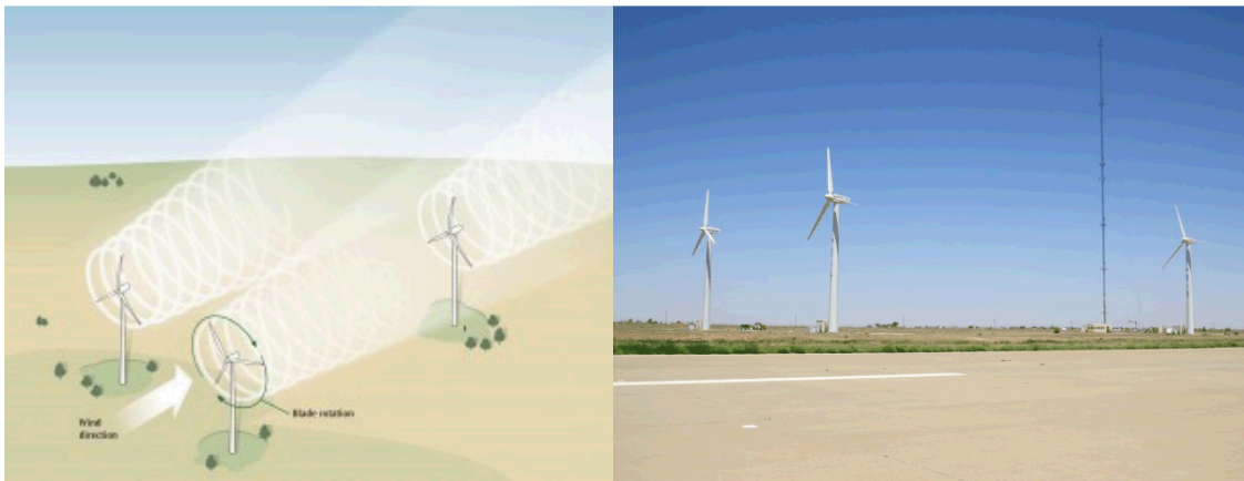
Figure 1. Turbine-turbine interaction schematic with wakes denoted by white helices and white fog (left). SWiFT Facility (right).
