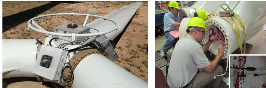
Figure 4. Rotor instrumentation data acquisition system (left) and rotor blade fiber optic instrumentation (right).
