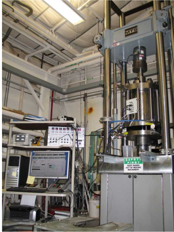
Figure 2. Testing system used to conduct cyclic load triaxial compression tests.
