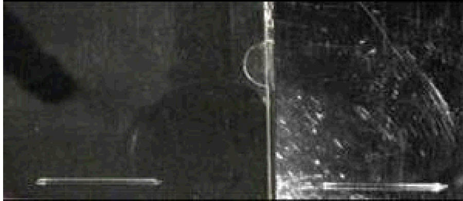
Figure 4: Images of CD jewel case under visible (left) and 365 nm UV light (right) [10].
