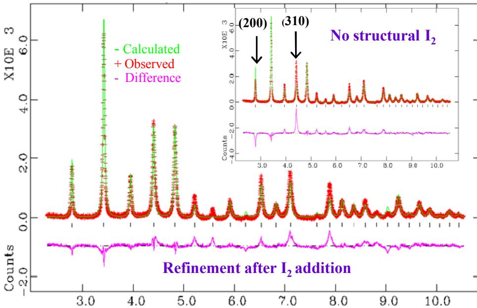
Calculated, observed and difference spectrum of  $0.4 \text{ I}/\text{Zn}$  loading of  $\text{I}_2$ @ZIF-8 after  $\text{I}_2$  inclusion in structure refinement by Rietveld analysis (inset: before  $\text{I}_2$  inclusion).
