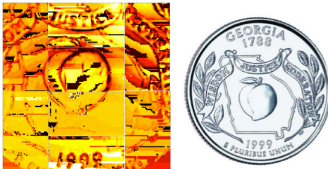
Figure 12. (a) 2D plot of the difference frequency between the Fabry-Perot modes of the transceiver when the emitted radiation is focused to a spot and reflected off a Georgia quarter which is scanned in the focal plane.
