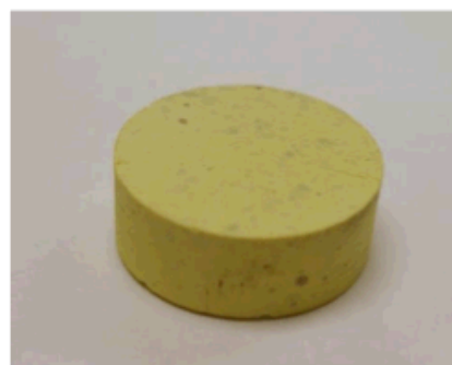
50 wt% AgI/50 wt% Glass 500°C for 3 hr
