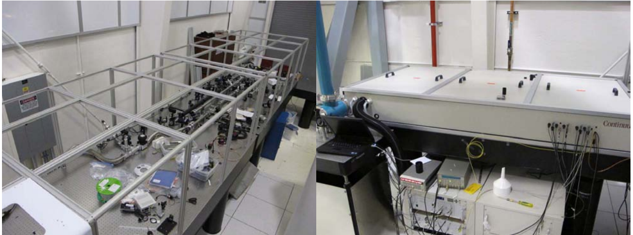
Figure 3. (left) Spatial filter/transport telescopes in place for signal and pump beam of all 4 OPA stages; (right) 5.5 J, 532 nm, 2 Hz pump laser source.
