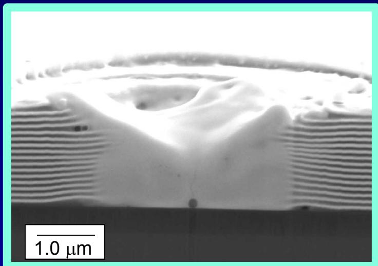
Reaction zone could be solely the result of laser Irradiation
