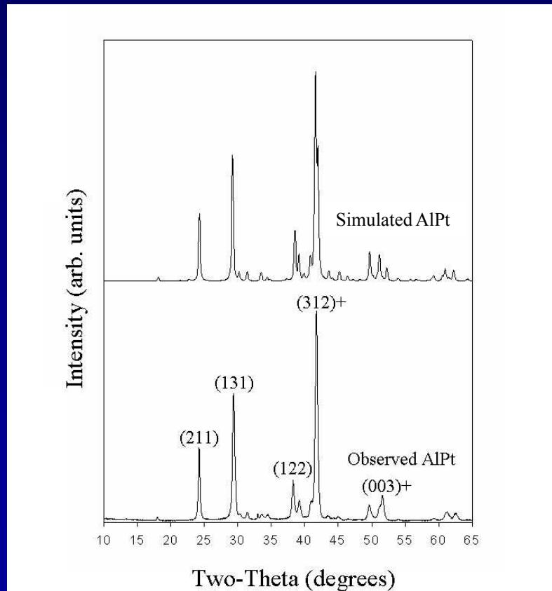
$\text{Al}_{0.5}\text{Pt}_{0.5}$  is cubic (FeSi structure) under equilibrium conditions but rhombohedral as reacted film.
