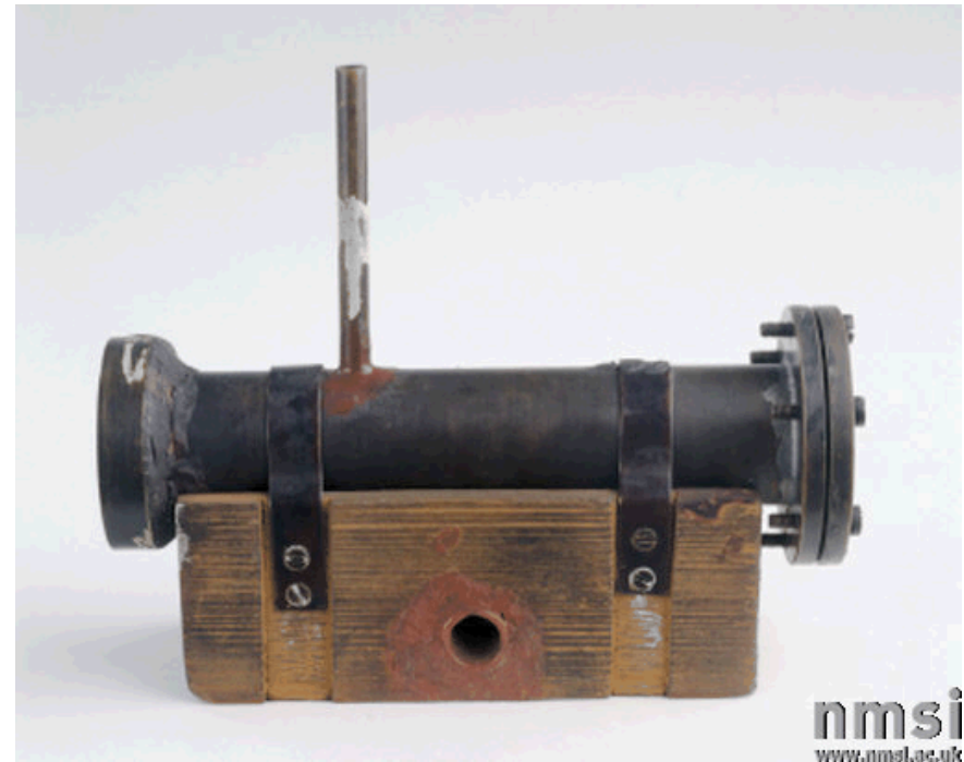
Chadwick's neutron generator: Polonium alpha source striking Beryllium target
