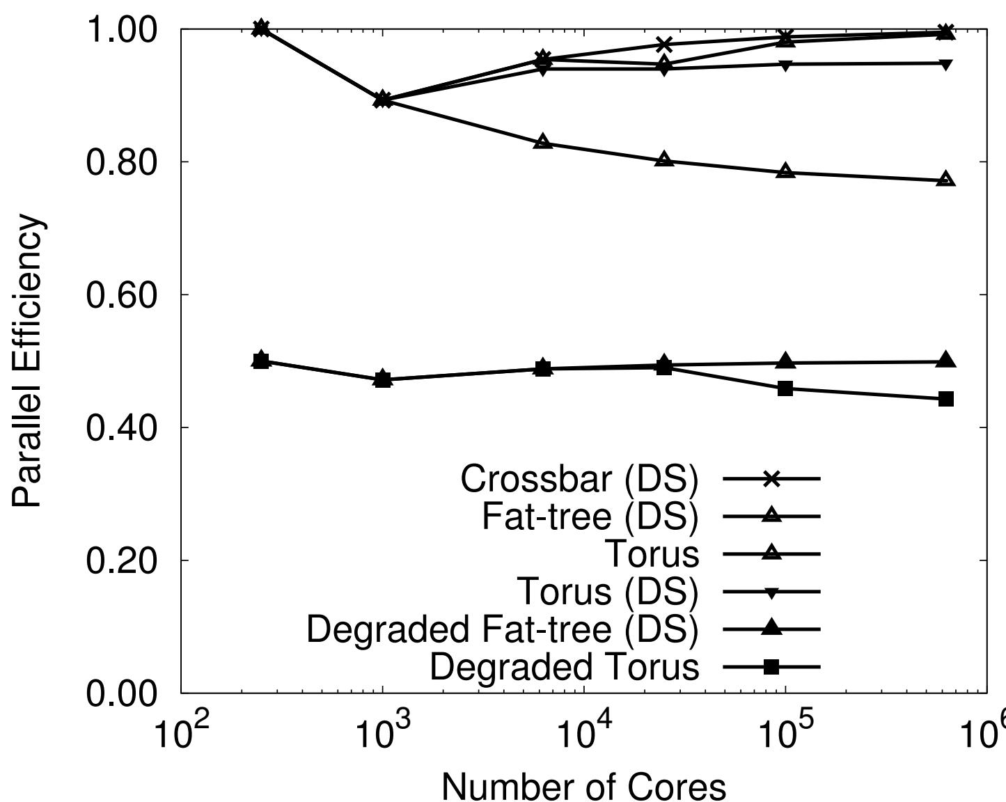
Weak scaling parallel efficiency of the systolic matrix matrix algorithm: 1) full crossbar network (DS), 2) fat-tree with radix 36 switches (DS), 3) 2D torus network, 4) 2D torus network (DS), 5) fat-tree with radix 36 switches with a single degraded node (DS), 6) 2D torus with a single degraded node. DS designates use of the direct send algorithm.
