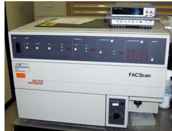
This old (c. 2000) FACScan analyzes 20,000 cells/s with 5 fluorescence and 2 scatter channels
