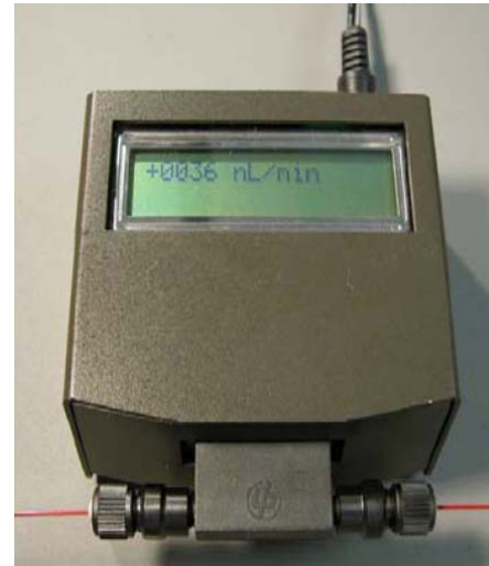
Commercial nanoliter flow sensor with optional RS-232 interface to PC
