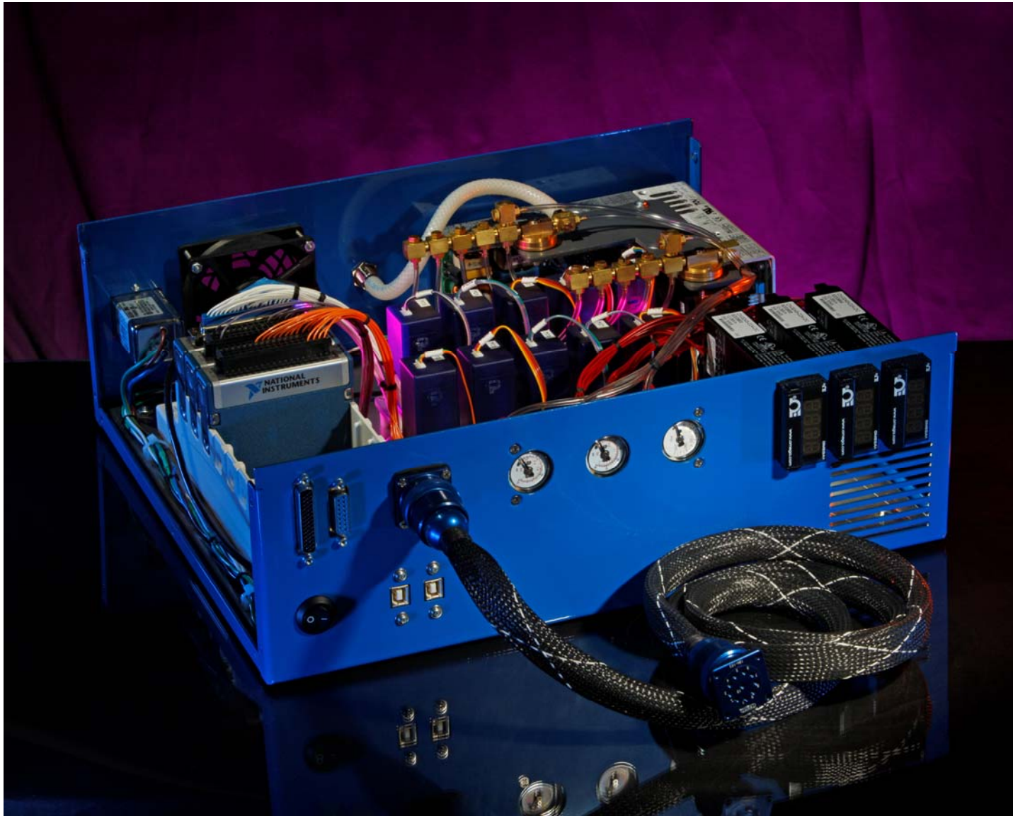
Integrated benchtop chip controller package consisting of multiple-range pressure controllers, 3 independent temperature controllers, and data acquisition/signal processing hardware. Hardware designed and built by: Ron Renzi, Jim Van De Vreugde, Mark Claudnic, Jerry Inman; Funding from Sandia LDRD; Photo credit: Randy Wong
