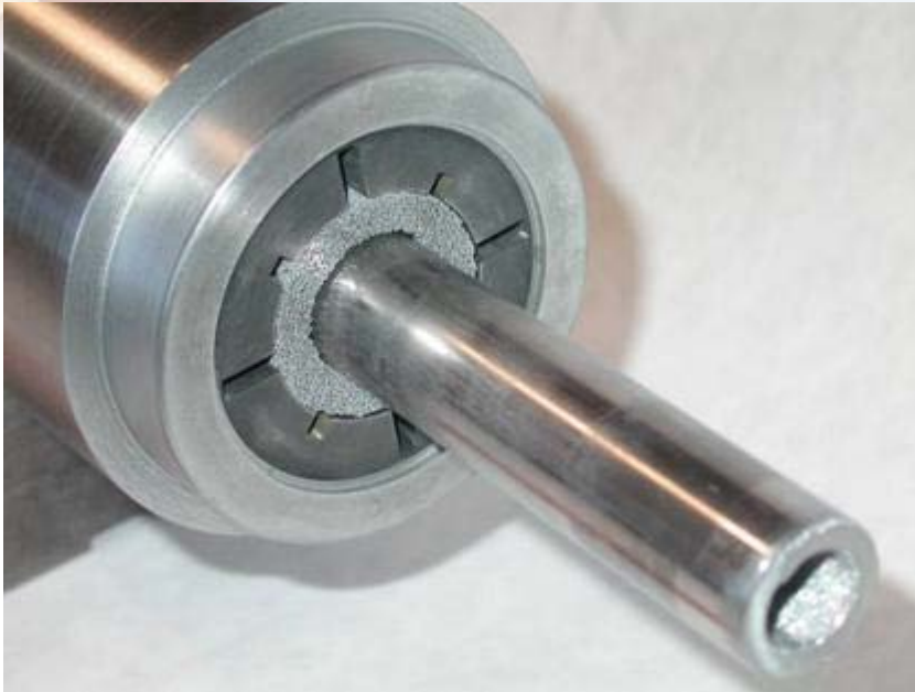
Views showing Mo Inner Tube + Mo foam fully slid into the ID of Mo
