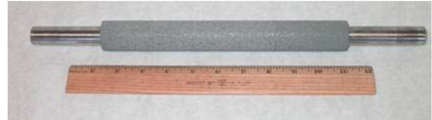
Mo foam heat exchanger slid over Mo inner Tube with dendritic internal coating
