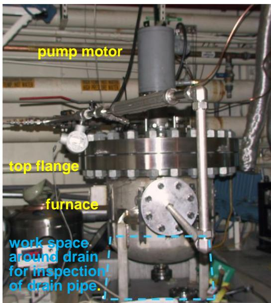
Fig. 2. LIMITS furnace and pump (above). Area indicated around drain was isolated by skirt so that a cover gas could be used when the drain pipe was opened for inspection.
