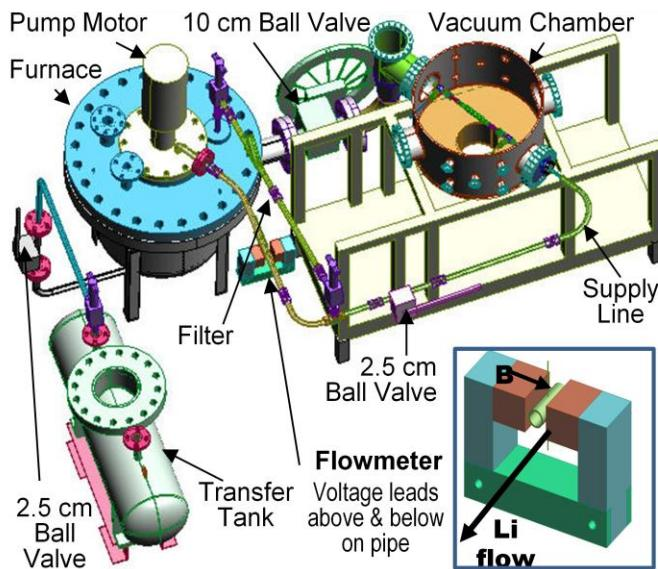
Fig. 1. Here LIMITS is configured to test a Li jet flowing across a vacuum chamber previously used with our small e-beam. Parts: lithium furnace with rotary pump, heated piping, heated transfer cask, and, for the NSTX test shown here, a nozzle and flow collector. The e-gun and its vacuum system are not shown to reveal base of vacuum chamber.
