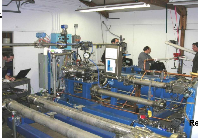
Heated Unrecuperated Brayton Loop
