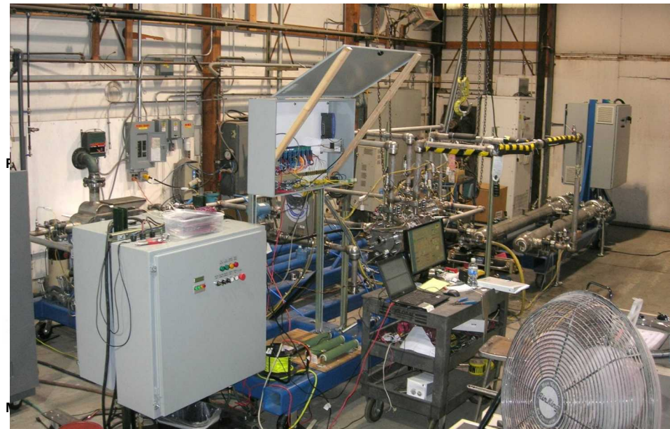
Split Flow Recompression Brayton Loop at Barber Nichols
