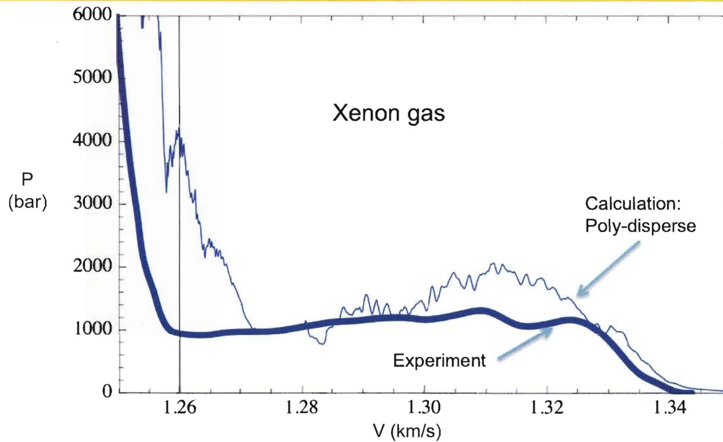
Thick curve: Xenon gas experimental data. Thin curve: calculation assuming a viscosity of  $186 \mu \text{ Pa}\cdot\text{s}$  and a distribution of particle diameters in the ratios  $0.1[0.2 \mu\text{m}] + 0.1[0.3 \mu\text{m}] + 0.1[0.4 \mu\text{m}] + [0.1[0.5 \mu\text{m}] + 0.5[1.0 \mu\text{m}]]$ .
