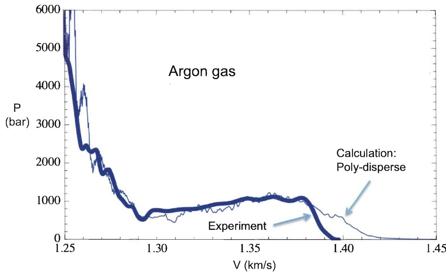
Thick curve: Argon gas experimental data. Thin curve: calculation assuming a viscosity of  $100 \mu \text{Pa}\cdot\text{s}$  and a
