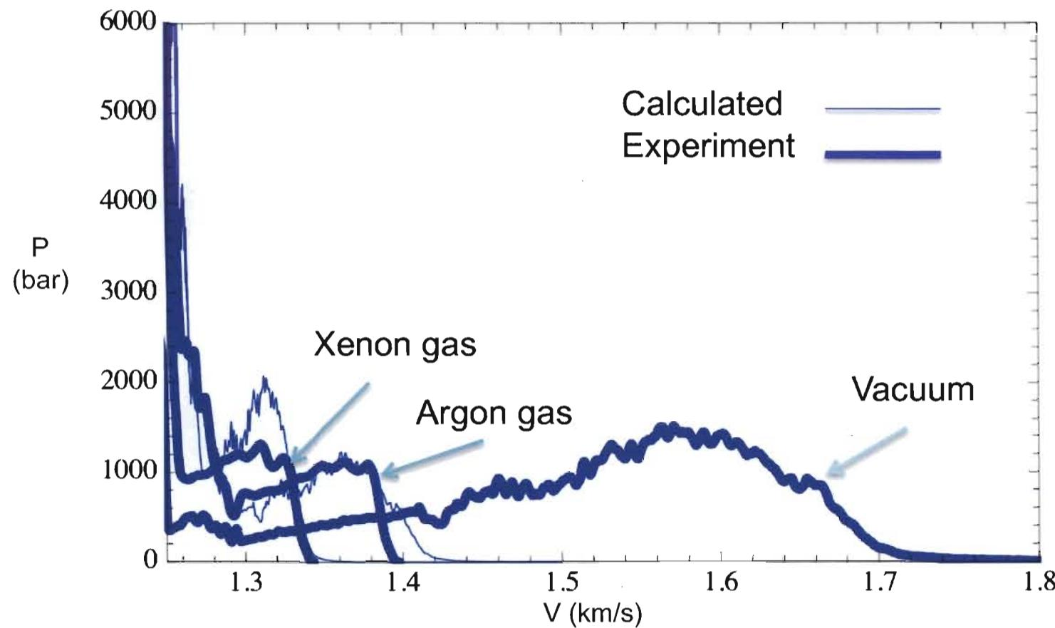
Summary of W vacuum and gas transport data and calculation assuming Stokes drag and spherical particles.
