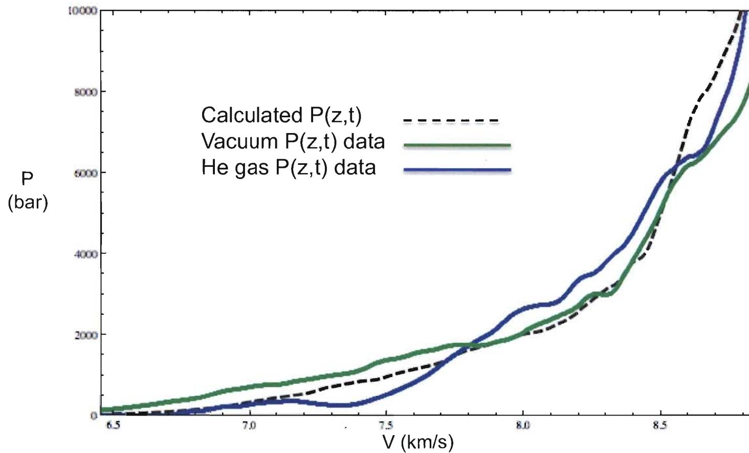
Data for Sn with a  $60 \mu\text{-in}$  finish driven with a Taylor wave profile with a shock pressure of 33 GPa.
