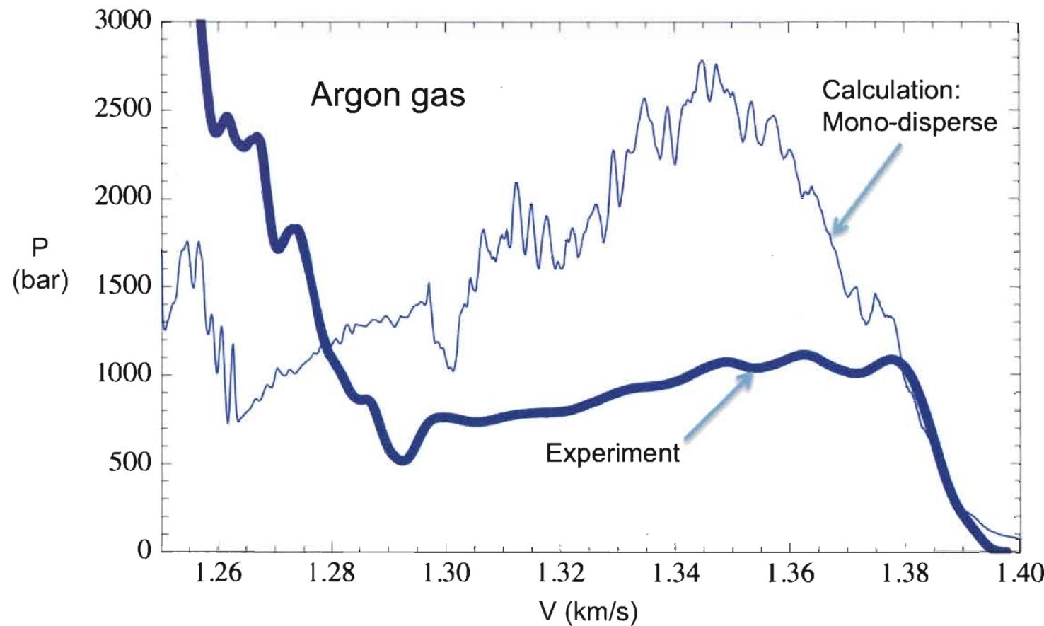
Thick line: Argon gas experimental data. Thin line: Calculation assuming Stokes drag using  $t_0=9.0 \mu\text{s}$
