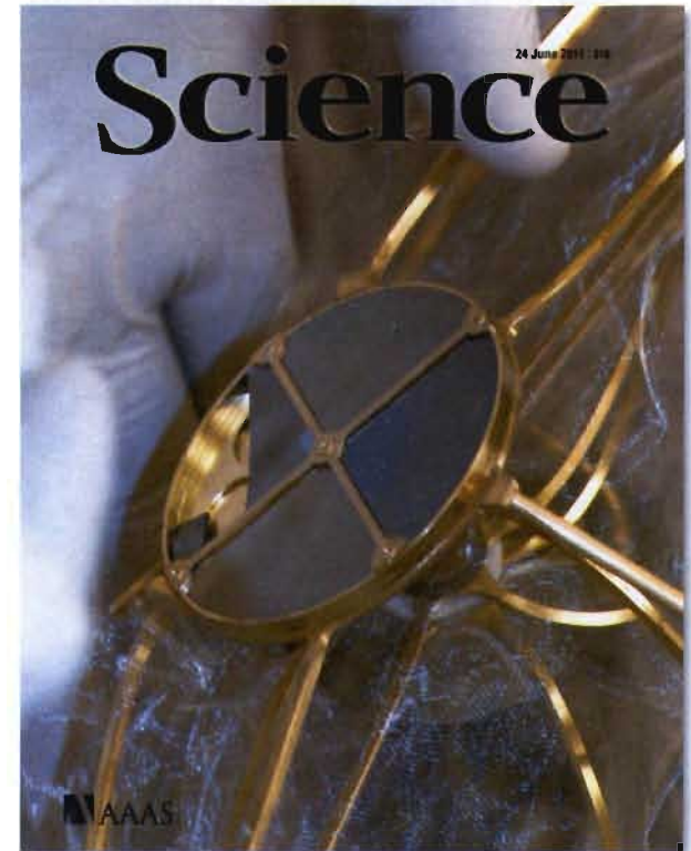
The Genesis Concentrator target after the crash of the sample return capsule
