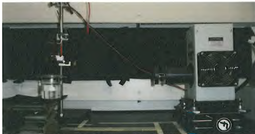
Figure 7. Photograph of the PEC testing setup in the fume hood. The solar simulator is on the right while the PEC cell is on the left.
