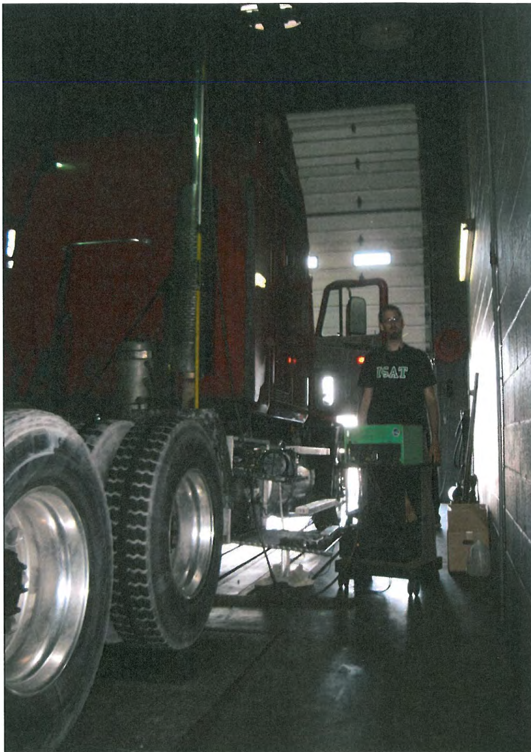
Figure 2: wider view of the 2003 Mack CX-600 semi-truck mounted to the Taylor TD-36 water-brake dynamometer. The emulsion system is visible in the center of the frame, beside the forward set of wheels. The device in the foreground to the right was used to measure particulate matter in the exhaust.
