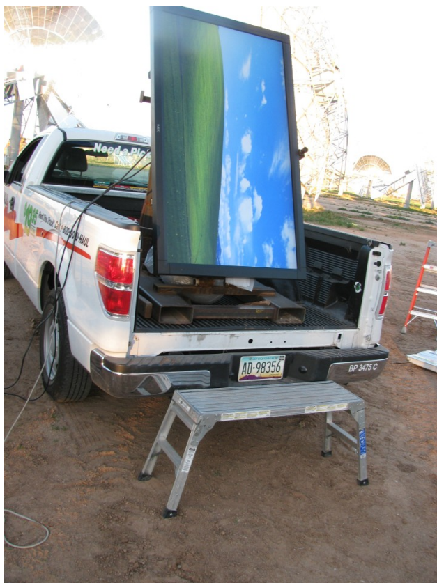
Figure 3. TRUCKFAST implementation of AIMFAST, with a monitor and camera mounted in a pickup truck. The monitor is angled to align a dish in the below-horizon “service” position.
