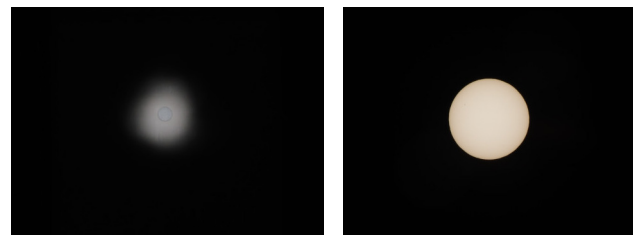
Figure 6. Images of the heliostat beam on the tower (left) and of the sun (right) taken with a Nikon D90. Both images were taken using the same camera settings (300 mm zoom, F/32, 1/4000 s). The sun image was taken using Tiffen neutral density filters.
