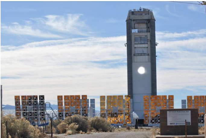
Figure 5. PHLUX testing using heliostats at the National Solar Thermal Test Facility at Sandia National Laboratories, Albuquerque, NM.
