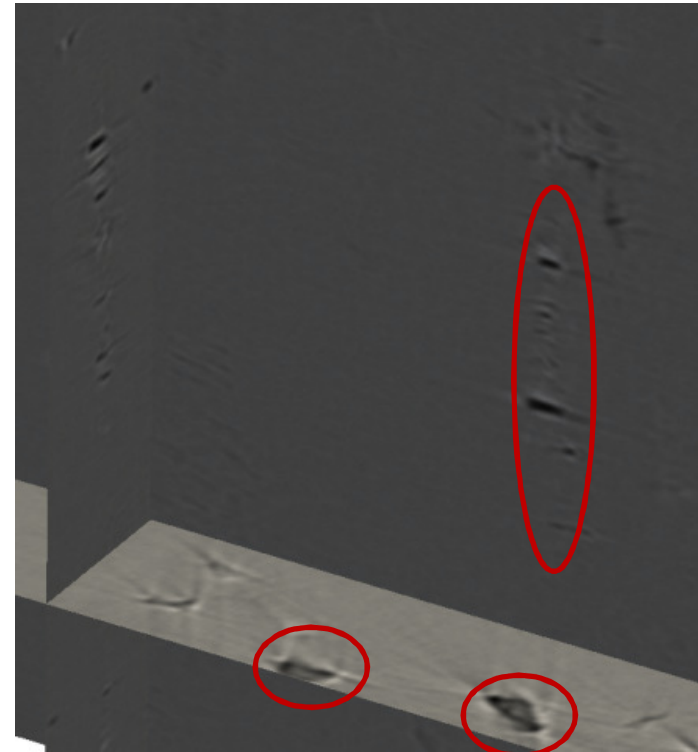
(b) Voids at the failure state
