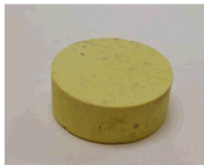
50 wt% AgI/50 wt% Glass 500°C for 3 hr
