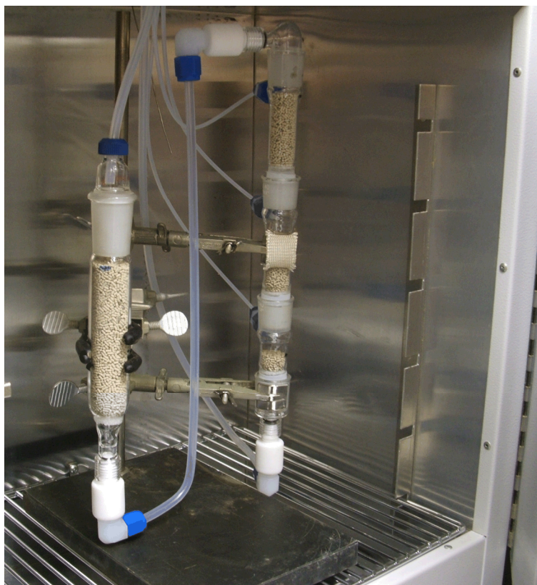
INL simulated dissolver off-gas setup
