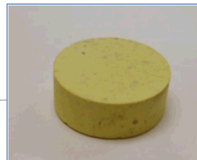
50 wt% AgI/50 wt% Glass 500°C for 3 hr
