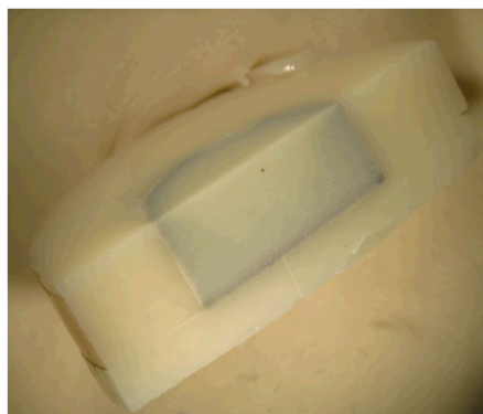
Glass shell, AgI/glass core 75/25
