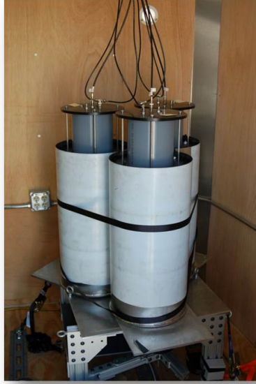
Figure 2. Left: The PRISM prototype, consisting of three large (27 L) liquid scintillator cells rotating around each other. As the system rotates, each cell is attenuated by the others for a given source location in azimuth. Right: The detected neutron rate (as simulated in MCNP) for a particular source location, where the three plots on the diagonal show the singles rate in each detector. These shapes are identical, but offset by a phase due to their different locations on the turntable. The off-diagonal plots show the rates of interactions in two cells as a function of turntable position; these events, however, are orders of magnitude less frequent.
