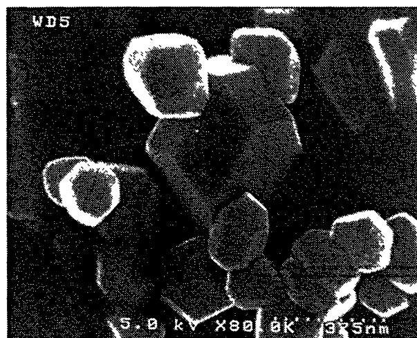
Figure 1a: Hydrothermally synthesized YAG:Tb powders (scale bar = 0.375 \mu\text{m} ).
