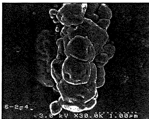
Figure 1c: Hydrothermally synthesized YAG:Tb grains from over-nucleated precursor gel (scale bar = 1 \mu\text{m} ).
