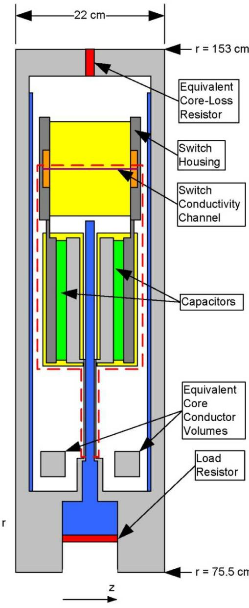
*A single LTD brick consists of two capacitors connected in series by a low-inductance switch. Forty bricks inside a low-inductance cavity, connected to a load and including ferromagnetic cores, comprise a single LTD cavity.*
