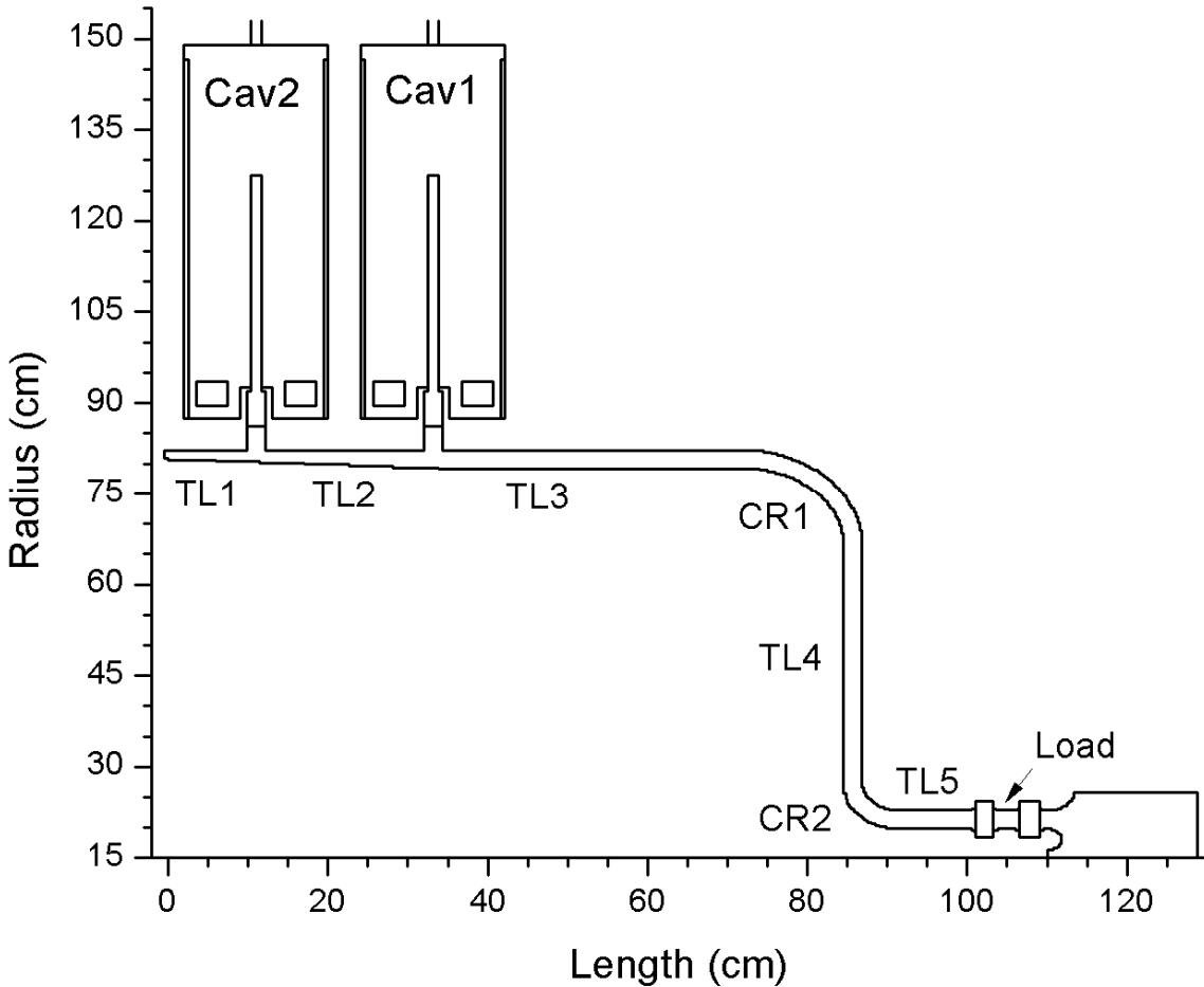
Cross-sectional view of a 2-cavity system model in Lsp. Such a model can be used to study field stresses in the Mykonos-2 accelerator.
