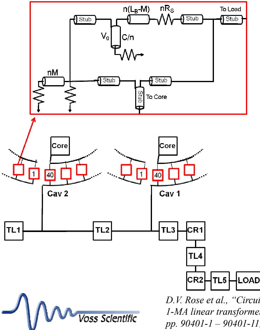
Circuit schematic of two LTD cavities driving a common water-filled coaxial transmission line terminated by a resistive load.
