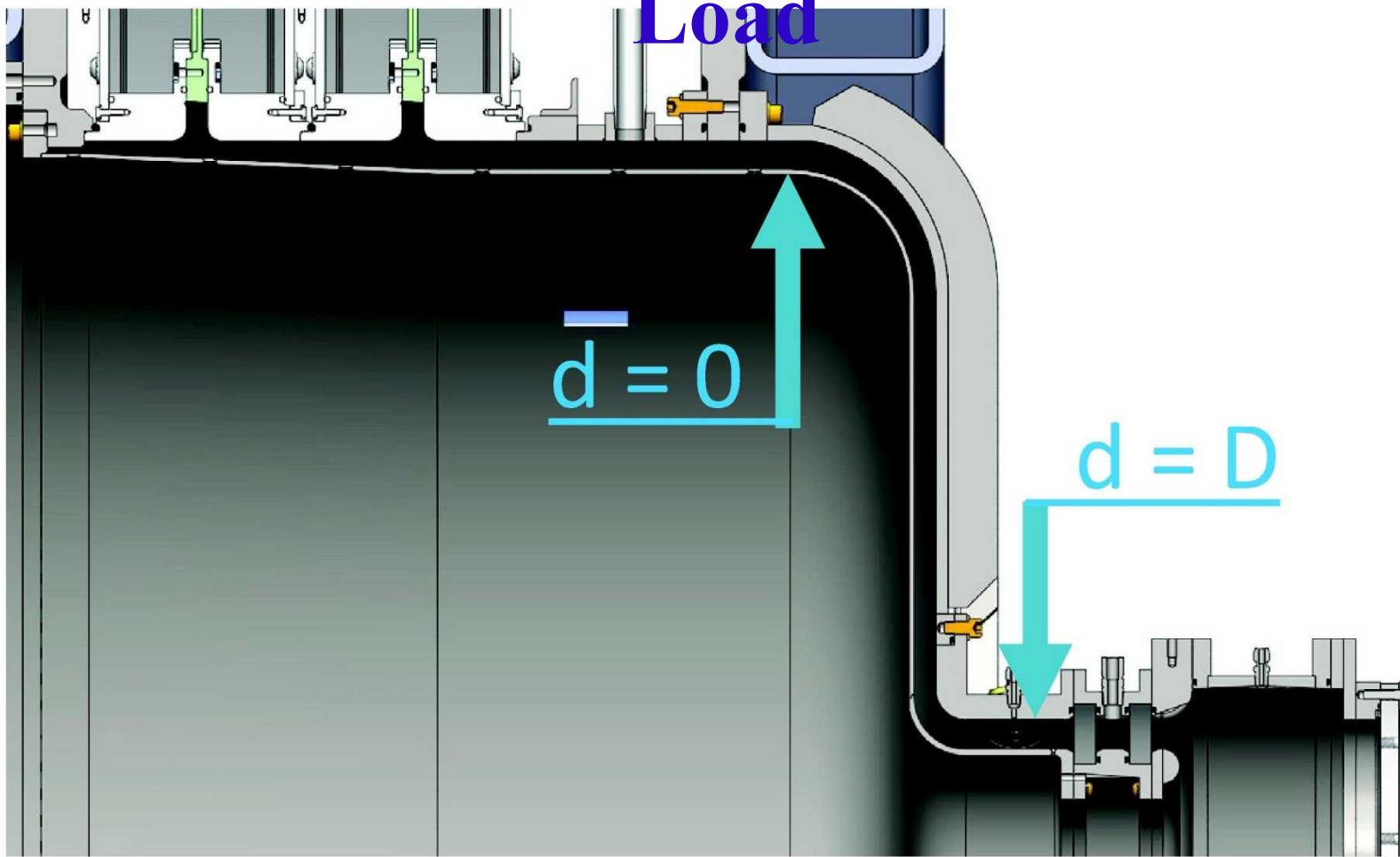
*The transmission line and load geometry for the Mykonos-2. Detailed modeling of the load is necessary to accurately produce reflections for the transmission line field structure.*
