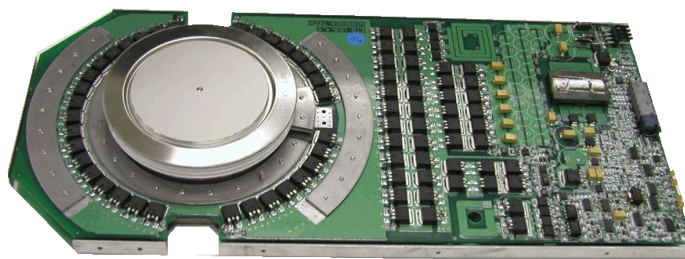
Figure 5. High-voltage silicon thyristor module co-developed by Sandia National Labs.
