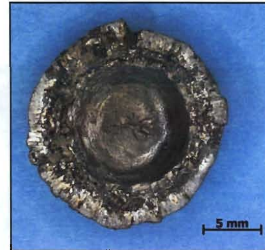
4000 ft/s (1220 m/s) Front of cover plate Fragment Impact Side
