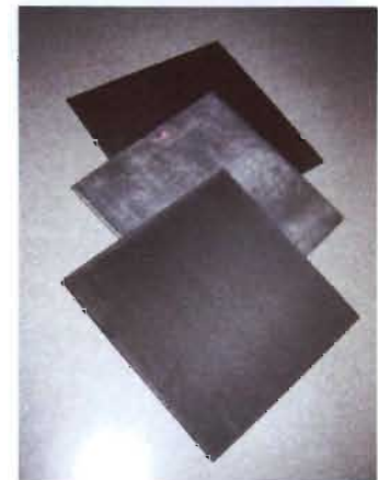
AISI 4130, Aluminum, Composite samples - AMRDEC
