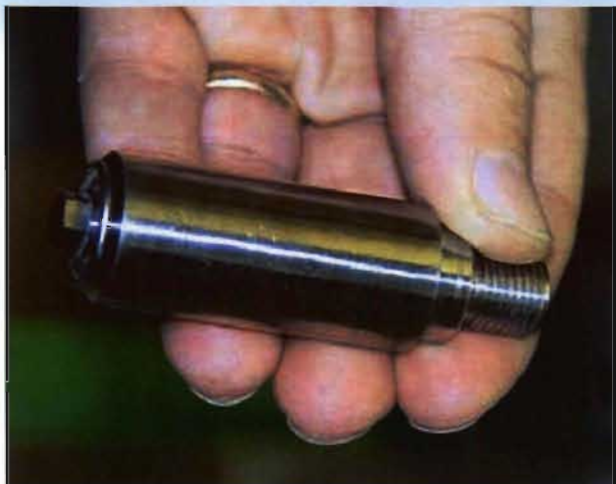
Photograph of an Am-Be neutron source used in well logging.
