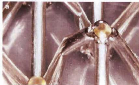
Buckling in hollow tube micro lattice structure
