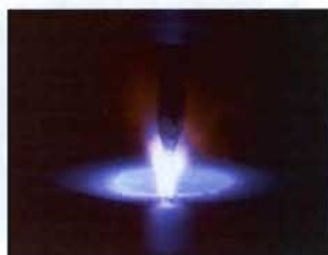
Electro-Static Discharge testing on PETN
