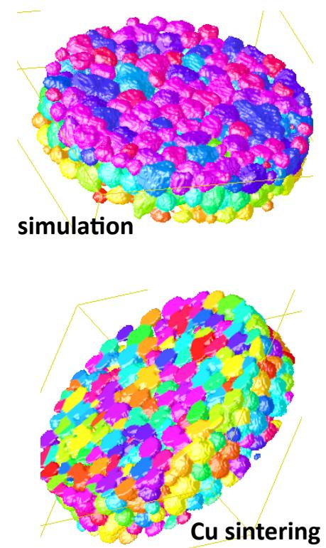
The GSD from simulated sintering is very similar to the 3D image of Cu sintering. Differences are due primarily to edge effects.
