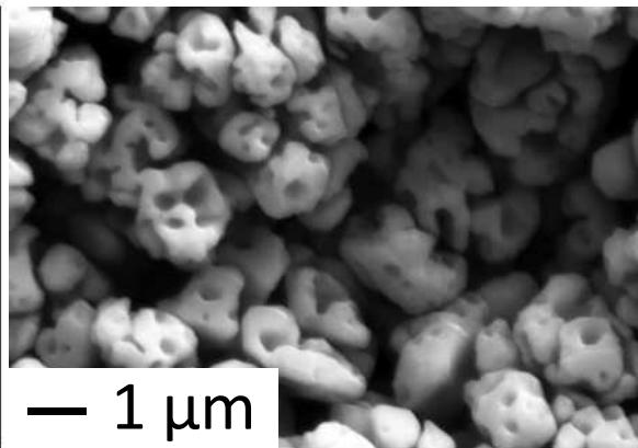
Partially irreversible copper plating on the electrode results in a lower coulombic efficiency. However this reversibility can be controlled by utilizing different anions.
