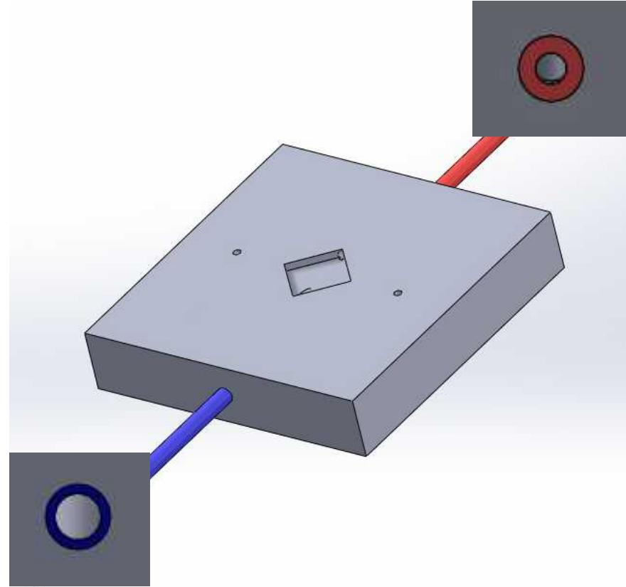
The back pressures from the viscous materials are minimized by increasing the outlet to inlet ratio and by smoothing the turns in the flow field.
