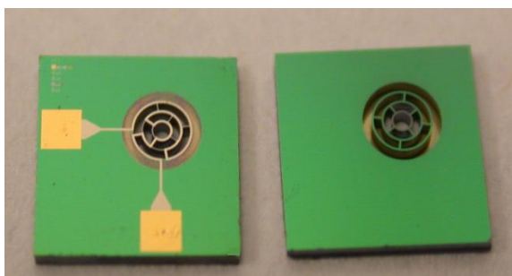
Hot Plate (Planar) Designs - Heater element on SiN membrane
