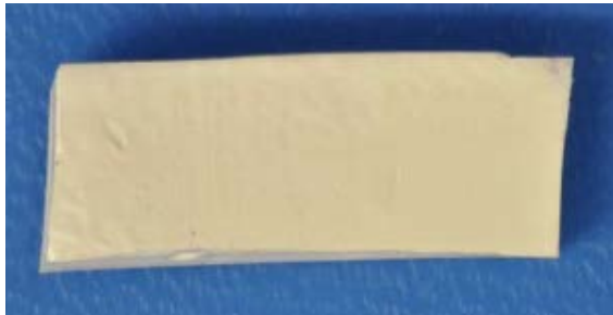
Doped 300 \text{mg}/\text{cm}^3 foam
