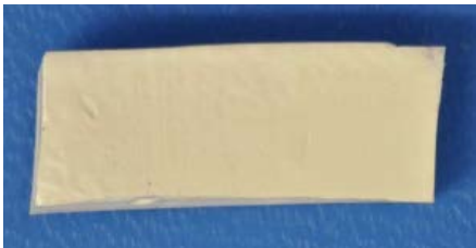
Optical image of 0.300 g/cm 3 PMP foam
