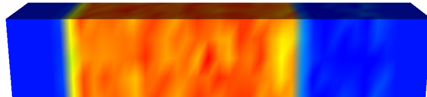
Compressive stress field for an atomic simulation of shock loading
