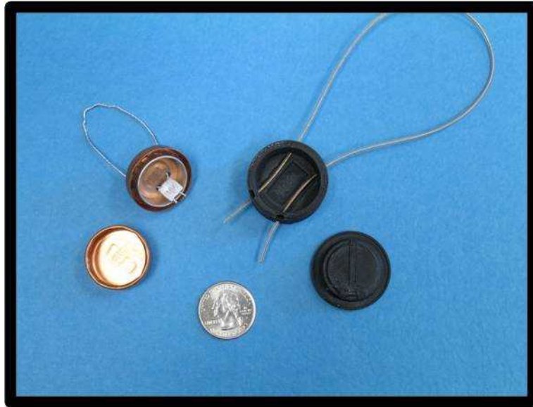
Figure 1: Size comparison of a metal seal (left), rapid-prototype mockup of the ITICS (right), and a U.S. quarter (bottom).
