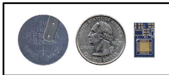
Figure 7: Battery and MCU board size relative to US quarter .
