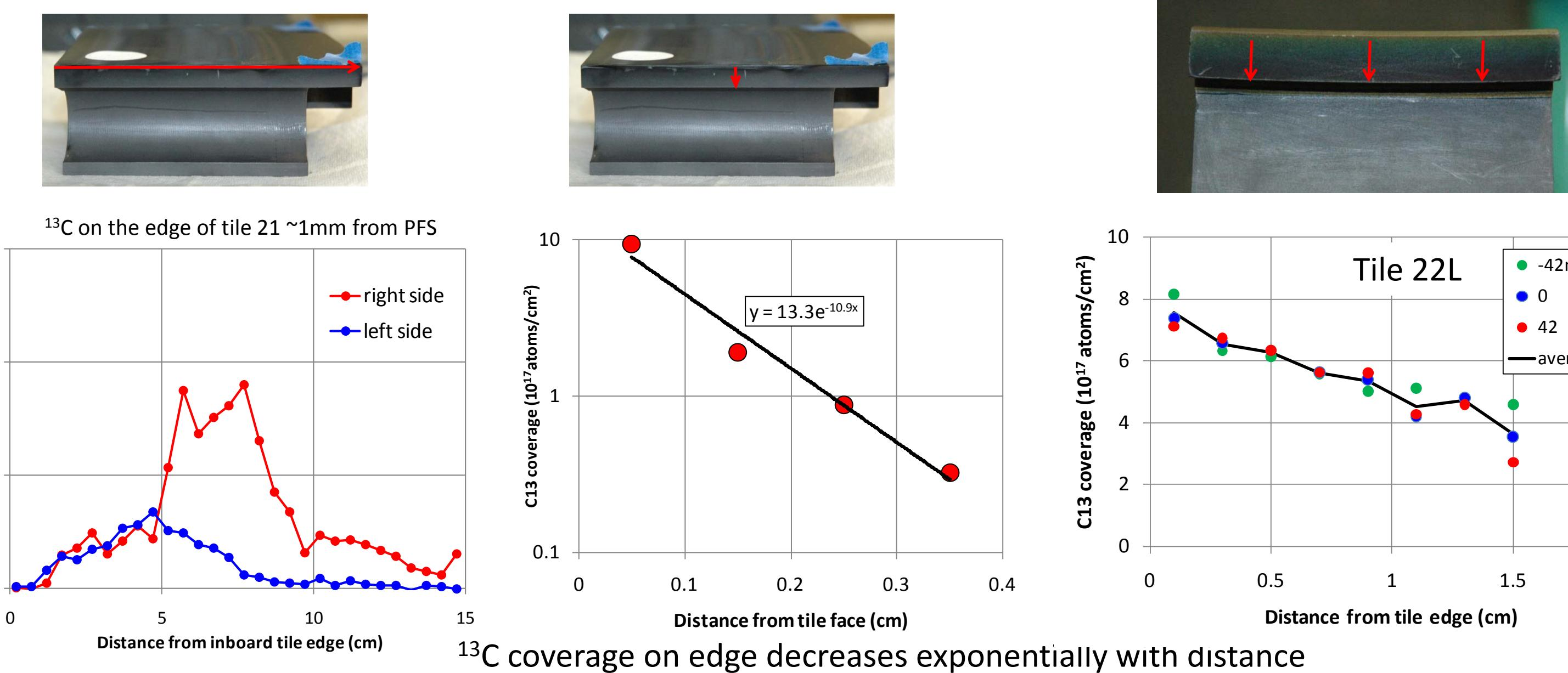
$^{13}\text{C}$  & D were also measured on the edges of tiles 1 & 21.
