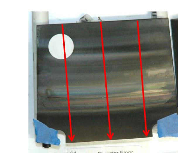
$^{13}\text{C}$  and D coverage measured along 3 poloidal scans on each of 37 tiles
