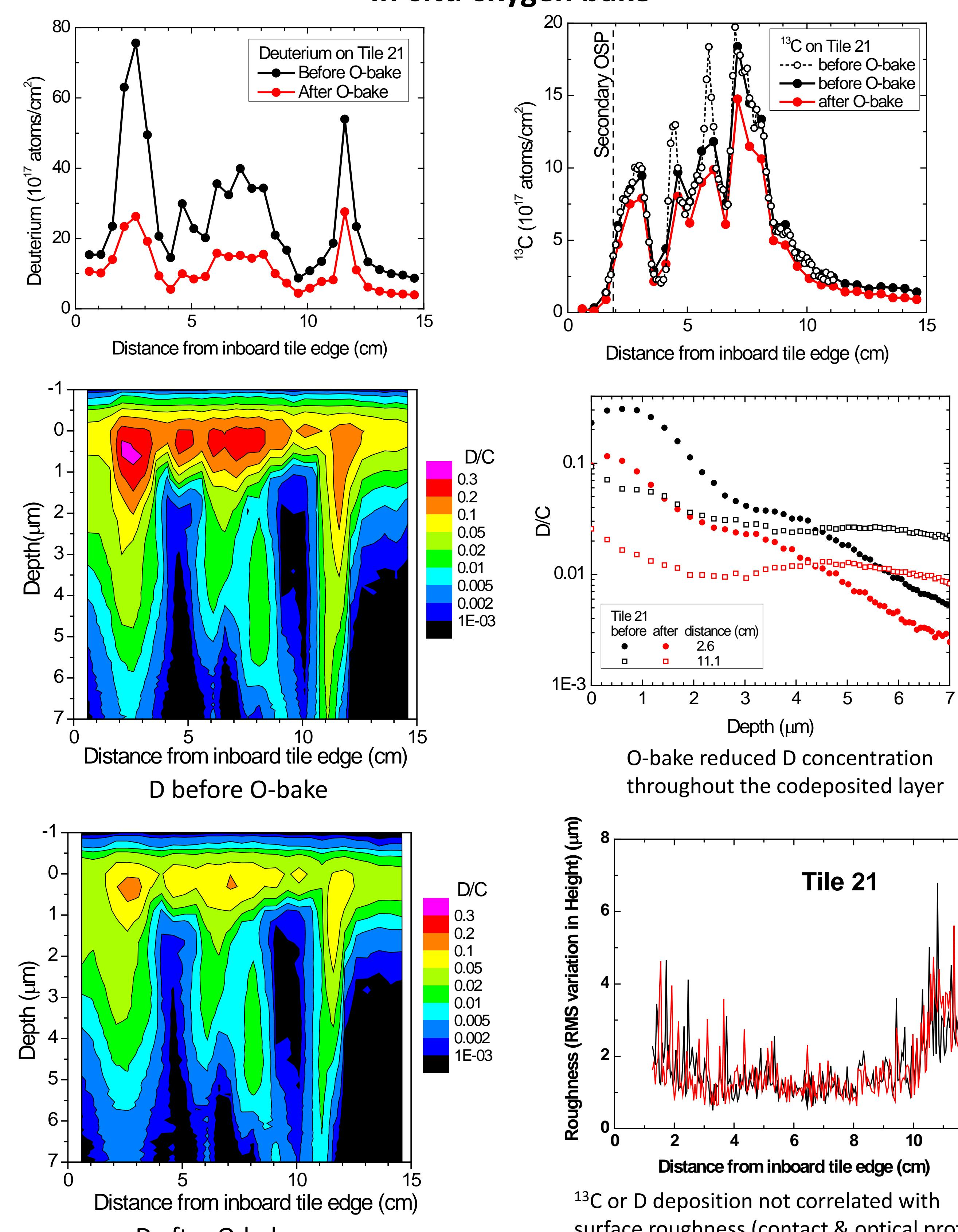
**NRA Measurements of  $^{13}\text{C}$  and D before and after oxygen bake**
