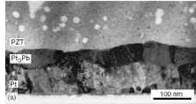
\text{Pt}_x\text{Pb} phase forms at the interface of the Pt electrode and the thin film. 5
