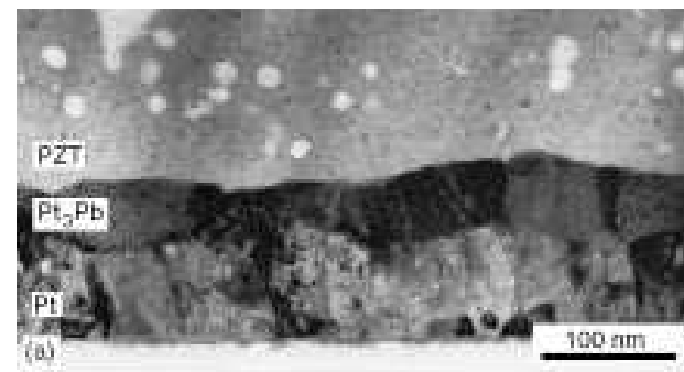
\text{Pt}_x\text{Pb} phase forms at the interface of the Pt electrode and the thin film. 5
