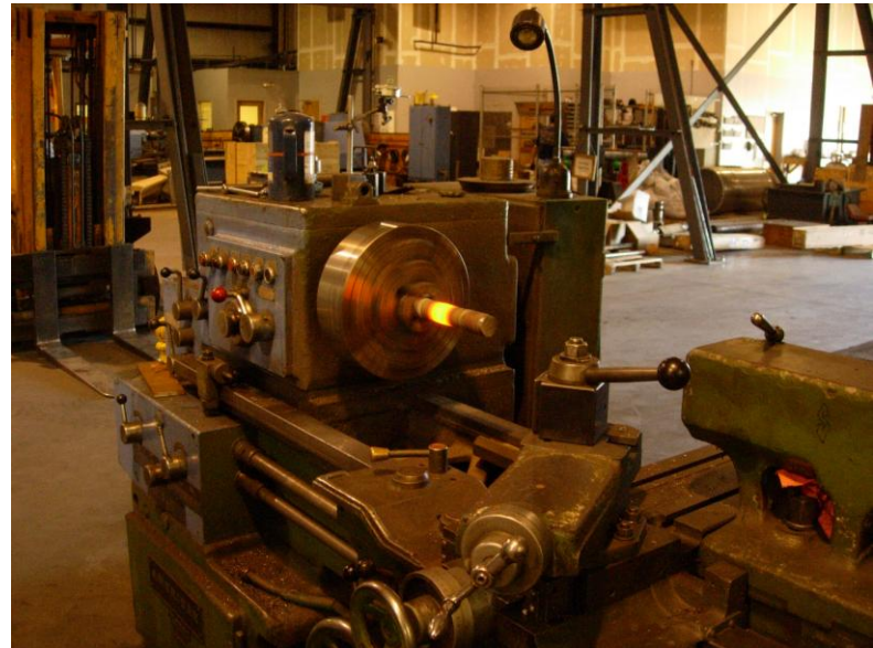
Application of fusible coating process at Thermal Spray Solutions facility
