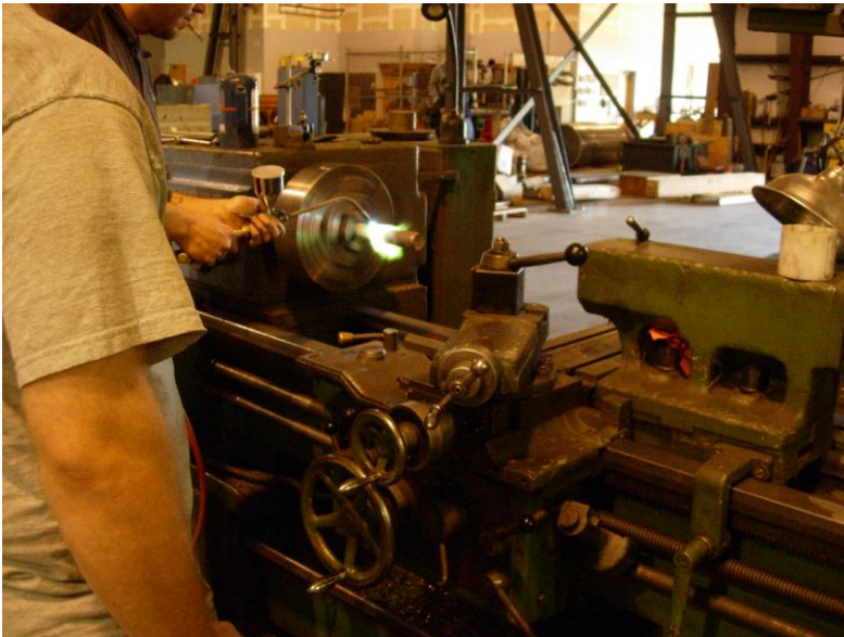
Application of fusible coating process at Thermal Spray Solutions facility
