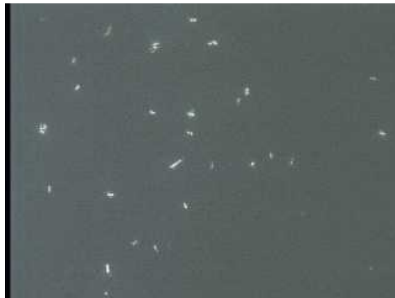
Pt/Au rods in 3% \text{H}_2\text{O}_2
