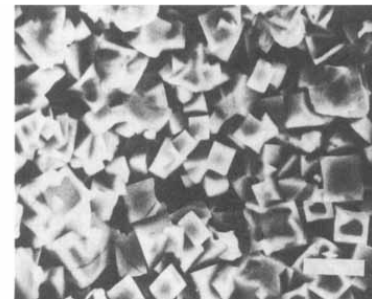
Fig. 2. Nasicon grain structure, showing intragranular microcracks (bar=10 μm).
