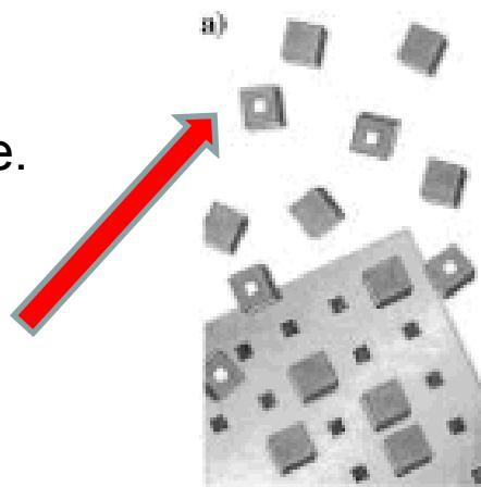
Au pads on a substrate are coated with an adhesive.
