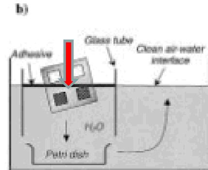
Die are held in place under water by the capillary forces of the adhesive, and the adhesive is then cured.
