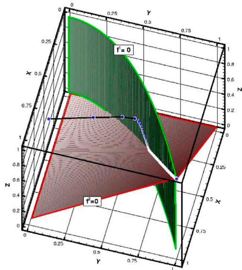
The CSP time integrator resolves the time scales on the order of the first active mode
