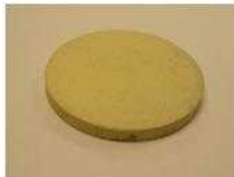
50 wt% AgI/50 wt% Glass, 500°C for 3 hr
