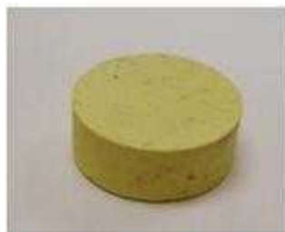
50 wt% AgI/50 wt% Glass 500°C for 3 hr
