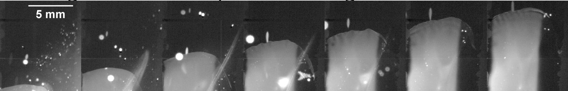
**5 mm thick NiTi foil, 30 nm bilayer thickness slows from 1.9 m/s to 0.9 m/s with quasi steady spin propagation**
