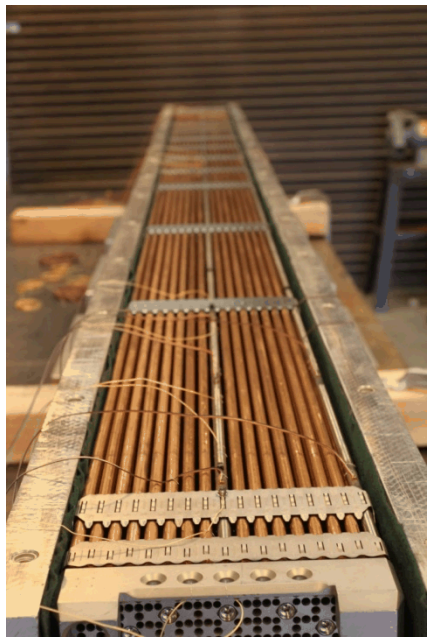
Figure 2. Diagram of Zircaloy-4 rods instrumented for the tests (top) and instrumentation on the actual assembly (bottom). The Zircaloy-4 rod shows as silver against the copper rods.
