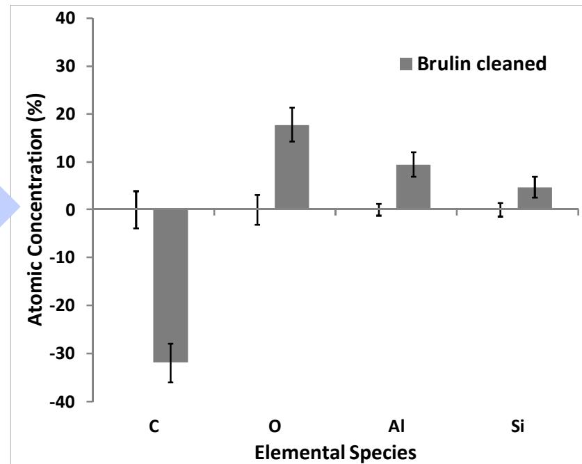
Brulin cleaning results in a significant decrease in carbon content at the surface (Auger results).
