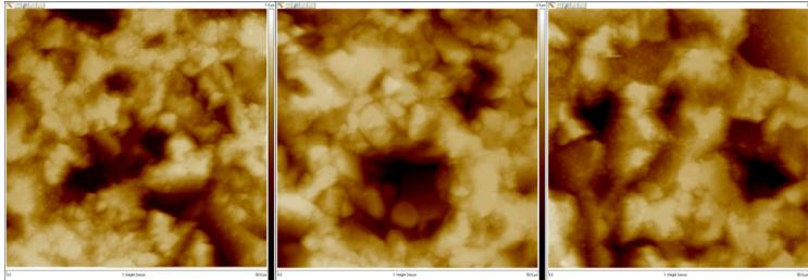
Brulin-cleaned Diamonite: roughness =  $1080 \pm 270$  nm
