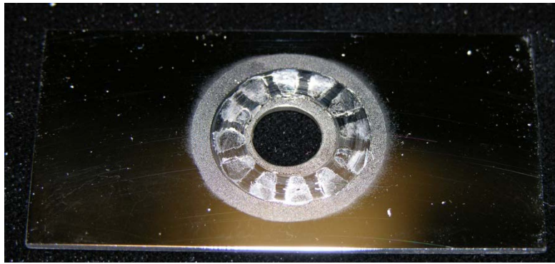
Figure 6: Hastelloy C-22 sample following long term exposure and removal of the MCA from the surface. Note the residual salt remaining on the surface, along with deposits from the PTFE tape which the MCA was wrapped with.
