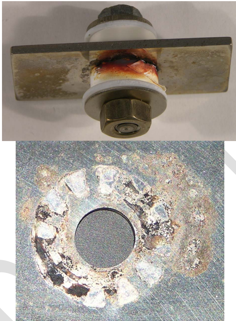
Figure 7: Crevice attack observed on 303SS samples after 100 days of exposure at a dewpoint of 94.5C and an ambient temperature of 101°C.
