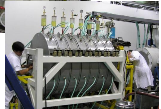
Seven-stage stack at the LTDR facility. Stacking cavities along their common axis adds voltages. This stack can deliver 1 MV to its load.
