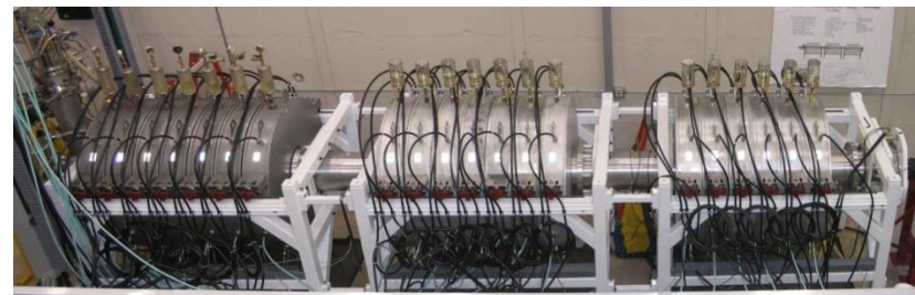
URSA Minor: a 21-stage linear stack, currently in verification phase. Rightmost cavity was under test when this picture was taken.
